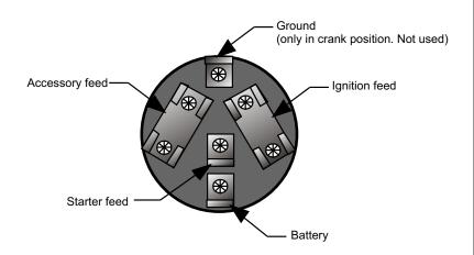
Connect the Ignition Switch wires as shown above.
